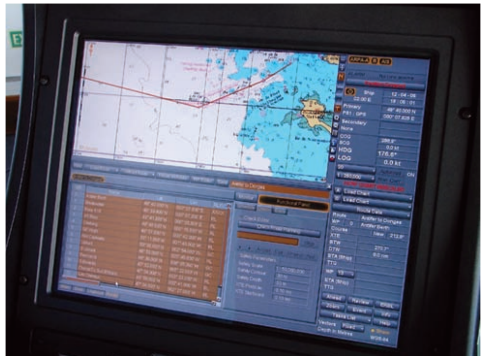
e-Navigation displays will integrate more information than is available with ENC’s today
